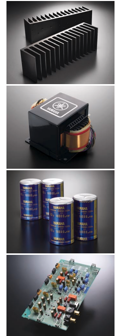
Large heat sink, huge power transformer, custom-made block capacitors (18,000µF) and preamp board.
